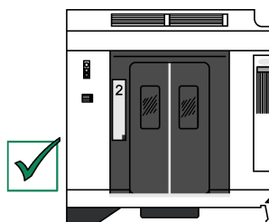
Figure B.3 — Example showing a compliant contrast area not exceeding 1,5 times the width of the door leaves and centred on the door
